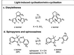
Fig. 1 Representative structures and photoisomerisation of most common classes of photoswitches applied in fluorescence microscopy.  $R_1-R_4$  indicate the most frequent substitution positions.
