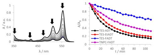
Fig. 2 (left) Absorption spectra of TES-ADT in CHCl<sub>x</sub> measured at timed intervals while under illumination from an LED desk lamp. (right) Normalised absorbance at  $\lambda_{max}$  for ADTs over time, while under illumination from an LED desk lamp
