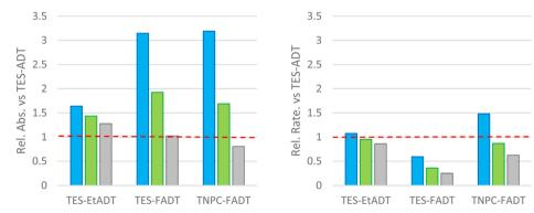
Fig. 3 (left) Integrated absorbance of ADTs versus light source spectra relative to the parent TES-ADT. (right) Relative reaction rates for photo-oxidation of ADTs using different coloured light sources, estimated from linear fits of absorbance over 10 minutes where  $A/A_0 > 0.9$ . All data relative to values determined for parent TES-ADT (depicted as the red line) with the same light source (blue, green, or white LED) and same concentration (3.3 µM in CHCl<sub>3</sub>)
