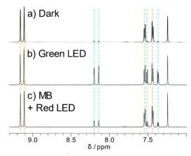
Fig. 5 Aromatic region of <sup>1</sup>H NMR spectra of TES-ADT (a) in the dark, (b) after white light irradiation and (c) with methylene blue and red light irradiation. All spectra measured in CDCl<sub>3</sub> at 298 K.
