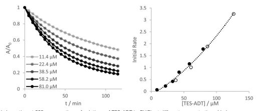
Fig. 4 Normalised absorption at 555 nm over time of solutions of TES-ADT in  $CHCl_3$  at different concentrations (darker = more concentrated) under illumination by green LED. (right) Plot of initial rate *versus* initial concentration. Filled circles monitored the first vibronic peak (555 nm) while the open circles were from a repeat experiment using the second vibronic peak (515 nm) allowing higher concentrations without saturating the detector.
