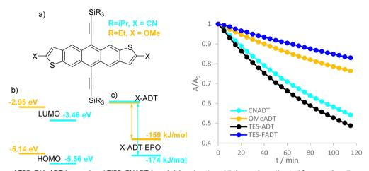
Fig. 7 (a) Structure of TES-OMeADT (orange) and TIPS-CNADT (cyan), (b) molecular orbital energies estimated from cyclic voltammetry, (c) computed reaction enthalpies for endoperoxide formation, (d) normalised absorbance of TIPS-CNADT and TES-OMeADT in CHCl<sub>3</sub> at 33 μM under irradiation by white LED. TES-ADT and TES-FADT (same conditions) are shown for comparison.
