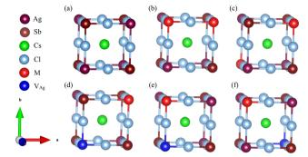
Fig. 1 Schematic models of the cubic unit of (a) the pristine Cs<sub>2</sub>AgSbCl<sub>6</sub> conventional cell, (b and c) configuration 1 with neighboring and distant M dopant atoms, respectively, (d) configuration 2, and (e and f) configuration 3 with a neighboring and distant M dopant atom and  $V_{Aq}$ , respectively.
