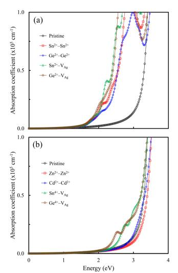
Fig. 6 (a and b) Calculated absorption coefficients of the pristine and all doped perovskites.
