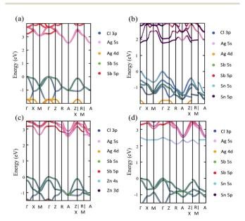
Fig. 4 Partial band structure of (a) the pristine perovskite, and the (b)  $\mathrm{Sn^{2+}}\mathrm{-Sn^{2+}}$ , (c)  $\mathrm{Zn^{2+}}\mathrm{-Zn^{2+}}$ , and (d)  $\mathrm{Sn^{4+}}\mathrm{-V_{Ag}}$  doped perovskites. Color codes are added to show the orbital contributions to the bottom of the CB and the top of the VB
