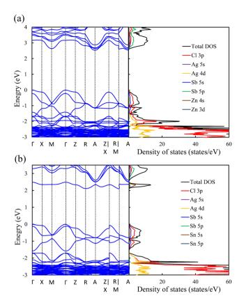
Fig. 5 Band structure (left) and density of states (right) of (a)  $Zn^{2+}-Zn^{2+}$ and (b)  $\mathrm{Sn}^{4+}\mathrm{-V}_{\mathrm{Ag}}$  doped perovskites.
