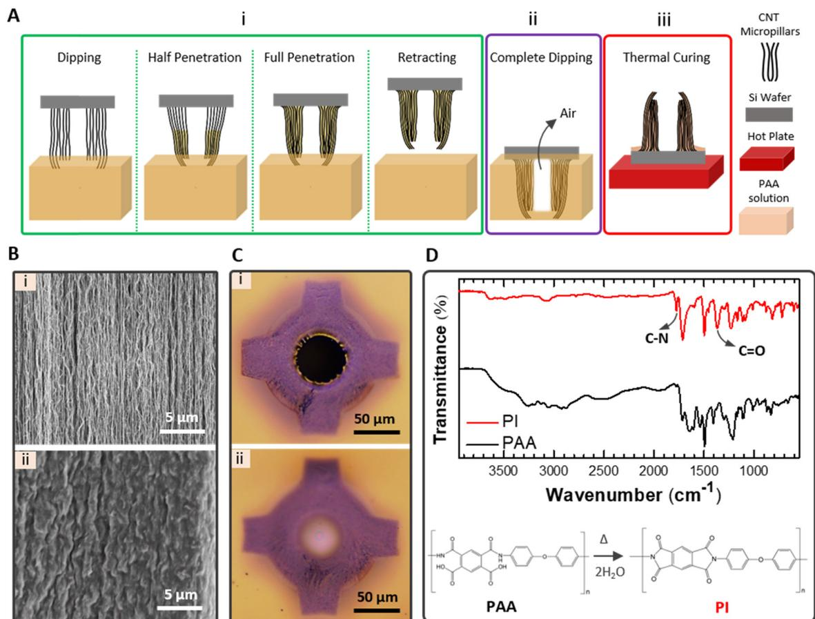
**Fig. 3** (A) Illustration of the PI reinforcement process of CNT-MN. (B) Magnified SEM images of the CNT microstructure (i) before (porous) and (ii) after (non-porous) PI reinforcement. (C) Bottom views of PI reinforced CNT-MNs with (i) dipping method (PI-free lumen) and (ii) spin coating method (blocked lumen with PI layer). (D) FT-IR spectrums of PAA and PI after thermal curing at 250 °C.
