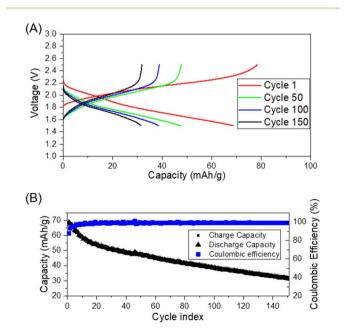
Fig. 4 (A) Room temperature galvanostatic charge—discharge plots of Li-ion cell using the gel polymer electrolyte containing 1BHETA:2PEG + 38% EMI-TFSI, LTO anode and LFP cathode; (B) coulombic efficiency and charge/discharge capacity of the same cell for 150 cycles.
