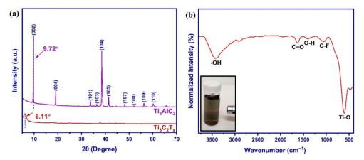
Fig. 1 (a) XRD patterns of Ti<sub>3</sub>AlC<sub>2</sub> and Ti<sub>3</sub>C<sub>2</sub>T<sub>x</sub>. (b) FTIR spectrum of Ti<sub>3</sub>C<sub>2</sub>T<sub>x</sub>. Inset in (b) shows the Tyndall effect of Ti<sub>3</sub>C<sub>2</sub>T<sub>x</sub> dispersion.
