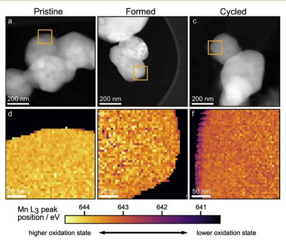
Fig. 6 EELS mapping of the Mn  $L_3$  peak position. (a–c), STEM-HAADF images of the *Pristine, Formed* and *Cycled*; orange squares outline the region where EELS mapping was conducted. (d–f), EELS mapping of the Mn  $L_3$  peak positions of *Pristine, Formed* and *Cycled* respectively. Colour schemes reflect the binding energy from low (lower oxidation state, dark purple) to high (higher oxidation state, yellow).
