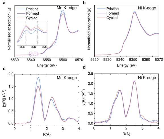
Fig. 5 XAS analysis on Li<sub>1.2</sub>Ni<sub>0.2</sub>Mn<sub>0.6</sub>O<sub>2</sub> structural changes. Evolution of XANES at the (a) Mn; (b) Ni K-edges. Inset in (a) shows an enlargement of the pre-edge features. Evolution of EXAFS at the (c) Mn and (d) Ni K-edges.
