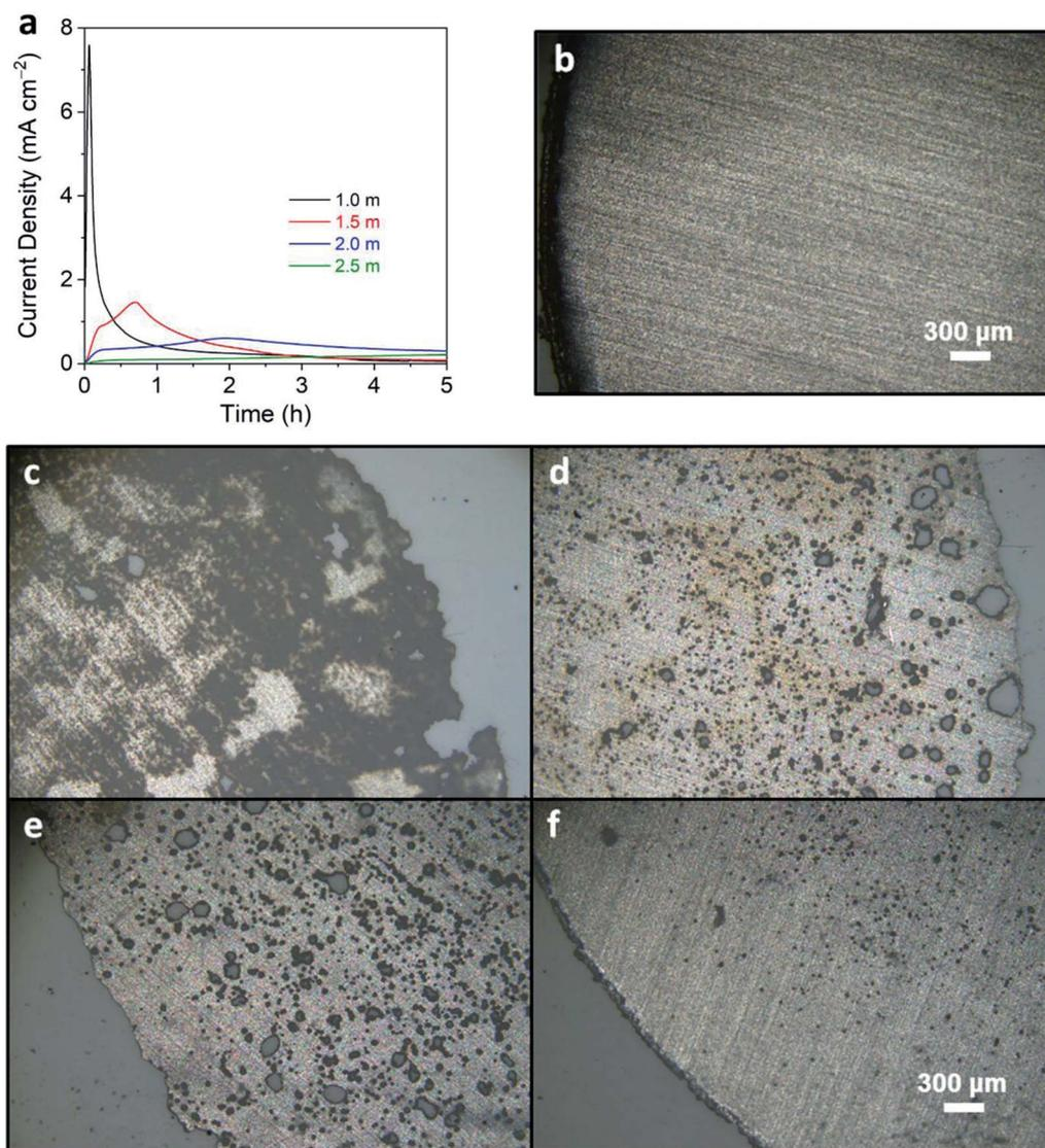
**Fig. 1** (a) Chronoamperometry curves with an imposed potential of  $4.5 \text{ V vs. Li/Li}^+$  for 5 h of aluminum current collectors when contacting 1.0, 1.5, 2.0, and 2.5 m LiTFSI in MPN electrolytes. Optical micrographs of (b) pristine aluminum, (c) 1.0, (d) 1.5, (e) 2.0, and (f) 2.5 m concentration after corrosion tests.
