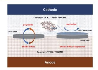
Fig. 1 Schematic illustrations of ZIF-7 modified separators for prohibiting the shuttling of redox mediators.
