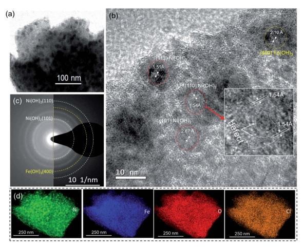
Fig. 2 TEM analysis of a Fe-18h/NF electrode: (a) TEM image showing  $\sim$ 10 nm diameter particles, and (b) HR-TEM image showing the dspacings with lattice defects on the (110) plane in the inset image. (c) SAED image showing diffused rings and dot patterns, indicating the coexistence of polycrystalline and amorphous phases. (d) HAADF mapping images showing the uniform distribution of the constituent elements.
