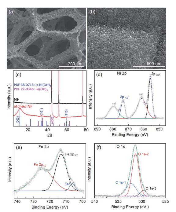
Fig. 1 SEM images of nickel foam (NF) etched for 18 h (Fe-18h/NF) in an ethanolic FeCl<sub>3</sub> solution at 50 °C: (a) surface view showing microporous Ni backbones at low magnification, and (b) a high-magnification view showing hierarchically-structured metallic Fe@Ni-Fe-hydroxide nanoparticles with a diameter of ~10 nm. (c) XRD patterns of pristine NF and NF etched for 18 h. XPS spectra of (d) Ni 2p, (e) Fe 2p, and (f) O 1s for the Fe-18h/NF sample.
