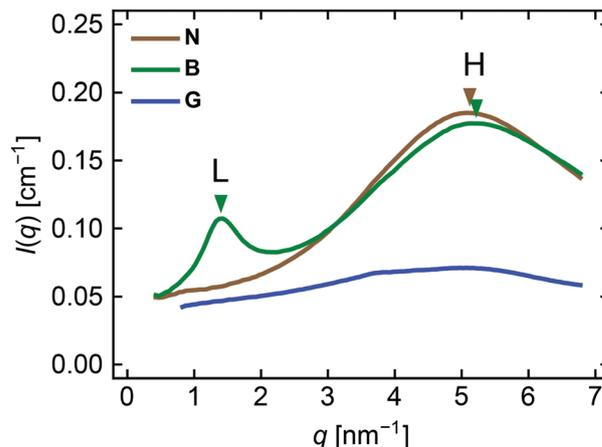
Fig. 4 1D SAXS profiles of the three networks at zero strain obtained by circular-averaging with the azimuthal angle  $\beta$  limited to  $45^\circ \leq \beta \leq 135^\circ$  and  $225^\circ \leq \beta \leq 315^\circ$ . The peak positions in **B** and **N** are indicated by triangles.
