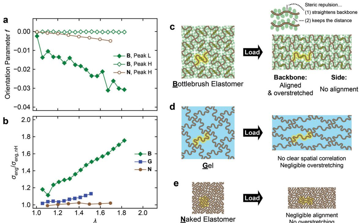
Fig. 7 (a) Orientation parameter ( $f$ ) measured by SAXS for peaks L and H of **B** and **N** and (b) the deviations from the nH model based on the uniaxial stress–strain data for the three networks. The first data point in each data series in Panel b has been omitted due to large error. (c–e) Schematic illustration of the structural changes in the three networks during uniaxial deformation.
