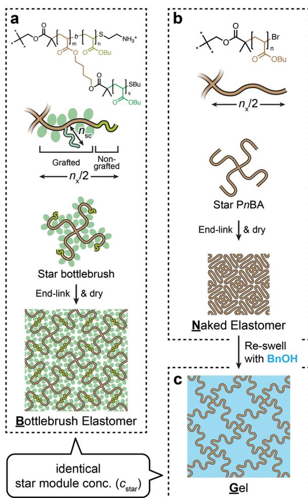
**Fig. 1** Preparation scheme for the three model networks used in this study. (a) Bottlebrush elastomer **B**. (b) “Naked” elastomer **N**. (c) Gel **G**. All three networks had almost identical polymerization degrees between cross-links ( $n_x$ ) by design. **G** was prepared so that the number density of the star polymer module ( $c_{\text{star}}$ ) was identical to that of **B**. The networks are illustrated in 2D for the sake of simplicity.
