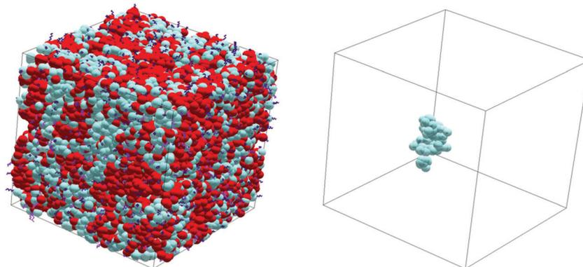
Fig. 2 Snapshot of an equilibrated sol for the s2020 system and one of the involved 800 molecules. Red and blue beads represent the segments on type-A and B prepolymers, respectively.
