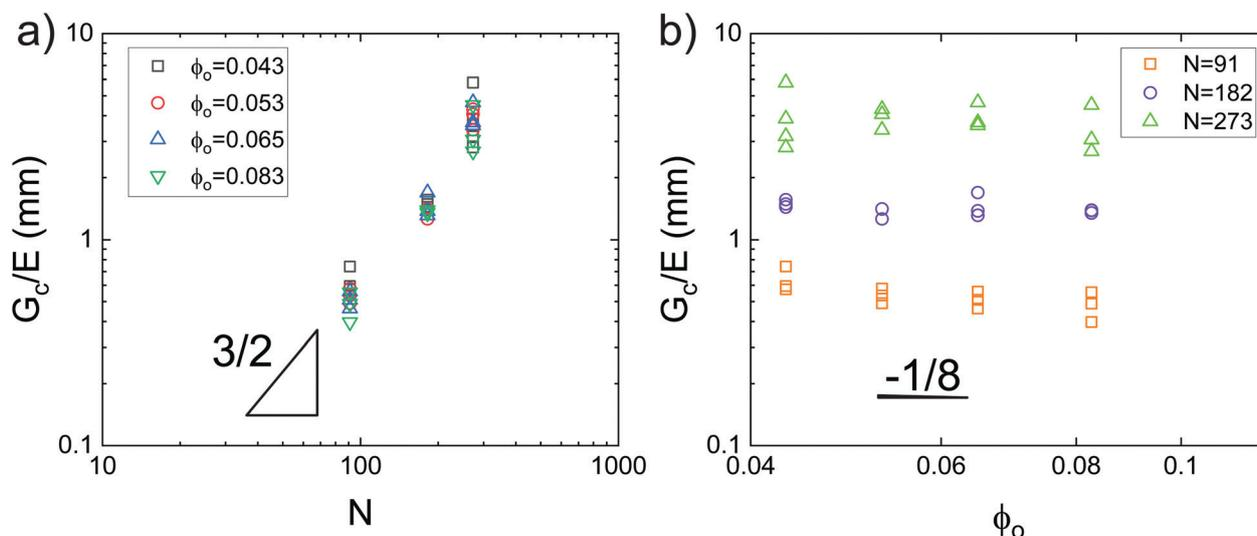
Fig. 2 Plots of the elastofracture length against (a)  $N$  and (b)  $\phi_o$  showing strong agreement with the scaling predictions of eqn (6). Data is taken from pure shear notch tests.<sup>16</sup> Agreement between the data and theoretical scalings shows that altering  $N$  is a more effective means of tuning  $G_c/E$ .
