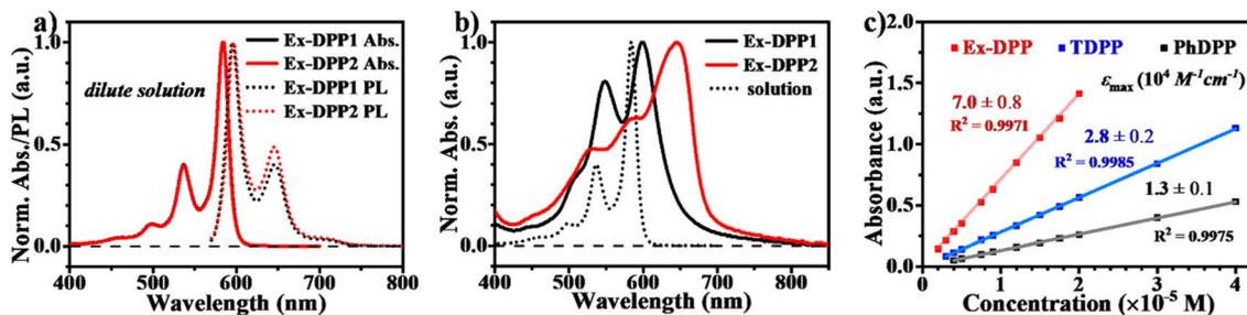
Fig. 3 Steady state absorption and PL spectra in (a) dilute CH<sub>2</sub>Cl<sub>2</sub> solution and (b) thin films of Ex-DPPs. (c) Extinction coefficient plot for PhDPP, TDPP and Ex-DPP (Ex-DPP1) molecules.
