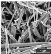
Fig. 2 (a) Standard sublimation reaction set-up. The quinone oxidant is placed in an outer 20 mL vial, whereas the copper salt, HHTP ligand, and solvent are placed in the inner 4 mL vial. As the reaction is heated, the quinone oxidant sublimes into the inner 4 mL vial. (b-d) Scanning electron microscopy images of  $Cu_3(HHTP)_2$  prepared with 3 equiv. of (b) 1,4-benzoquinone, (c) 2-methyl-1,4-benzoquinone, and (d) 2,6-dimethyl-1,4-benzoquinone.
