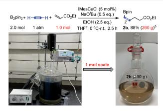
Scheme 4 Large-scale synthesis. <sup>a</sup>THF (3.0 L). <sup>b</sup>The purity of the product 2a is 86% after simple distillation and the reported yield is based on the pure product.
