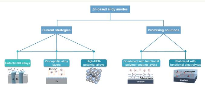
Fig. 4 The development of Zn-based alloy anodes for aqueous Zn batteries.
