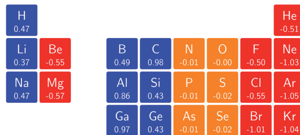
Fig. 6 Initial responses of the ionization energy in a magnetic field as a periodic table representation showing both the numerical values and categorising them with a color code in which blue indicates a positive derivative, red a negative derivative and yellow a derivative that is zero or close to zero.
