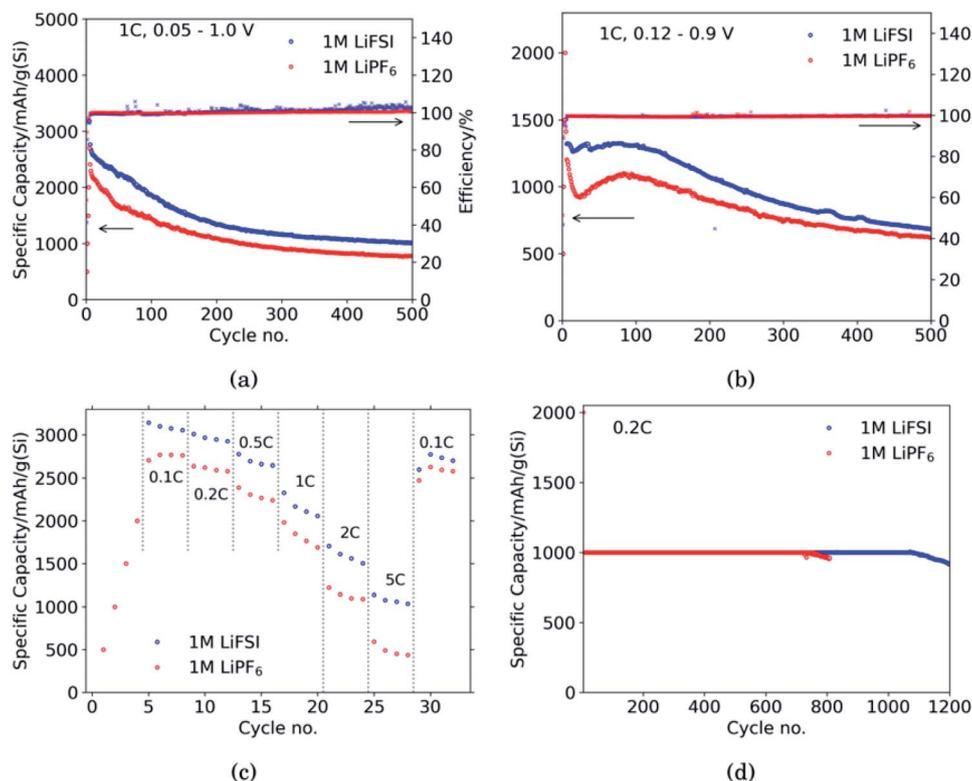
Fig. 1 Galvanostatic cycling tests comparing half cells with 60 wt% Si electrodes cycled in 1 M LiFSI (blue) or 1 M LiPF<sub>6</sub> (red). (a) Galvanostatic cycling in voltage range 0.05–1.0 V, (b) galvanostatic cycling in voltage range 0.12–0.9 V, (c) rate capability in voltage range 0.05–1.0 V, (d) galvanostatic cycling at 0.2C with lithiation of silicon limited to 1000 mA h g<sup>-1</sup> and delithiation to 1.0 V.
