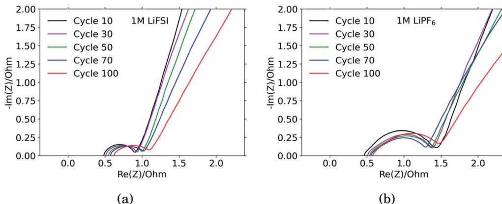
Fig. 4 Impedance spectra of Si electrodes cycled in (a) 1 M LiFSI and (b) 1 M LiPF<sub>6</sub>.
