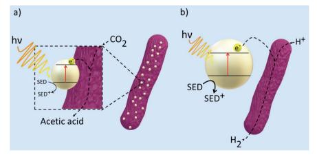
Fig. 5 General mechanism for electron transfer between a semiconductor and microbe in a hybrid photosystem. (a) Direct photoreduction of CO<sub>2</sub> to acetic acid in which the semiconductor is deposited onto the surface of the microbe (b) indirect photoreduction of CO<sub>2</sub> to H<sub>2</sub> by colloidal nanoparticles in the presence of electron mediators and SEDs.
