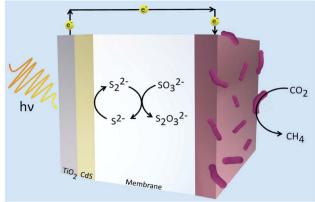
Fig. 4 Hybrid microbial photosystem designed by Xiao et al. consisting of a TiO<sub>2</sub>/CdS photoanode and a biocathode for CO<sub>2</sub> reduction to CH<sub>4</sub>.106 The sulfide electrolyte solution was used as sacrificial reagents to consume holes and prevent the corrosion of CdS.
