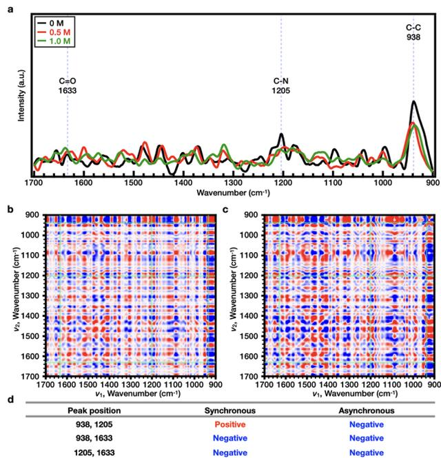
**Fig. 5** (a) Raman spectra of 10 wt% PNIPAAm solutions in D<sub>2</sub>O (black line), 0.5 M NaSCN (red line), and 1 M NaSCN (green line). 2DCOS (b) synchronous and (c) asynchronous spectra of PNIPAAm (10 wt%) with variation in the NaSCN concentration. (d) Peak descriptions for the 2DCOS results, where red is defined as a positive intensity, while blue is defined as a negative intensity.
