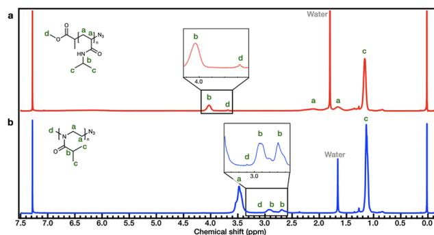
**Fig. 1** <sup>1</sup>H NMR spectra of (a) PNIPAAm and (b) PiPOx after purification in  $\text{CDCl}_3$ .
