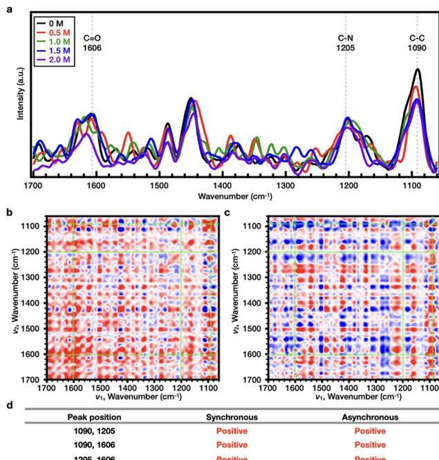
**Fig. 7** (a) Raman spectra of 10 wt% of PiPOx in D<sub>2</sub>O (black line), NaSCN 0.5 M (red line), NaSCN 1 M (green line), NaSCN 1.5 M (blue line), and NaSCN 2.0 M (purple line). 2DCOS (b) synchronous and (c) asynchronous spectra of PiPOx (10 wt%) depending on the NaSCN concentration. (d) Peak description of the 2DCOS result. Herein, red color is defined as a positive intensity, while blue color is defined as a negative one.
