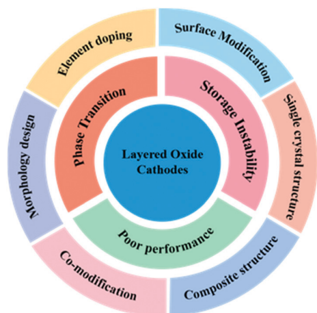
Fig. 1 Main challenges and solutions of SIB layered cathode materials.
