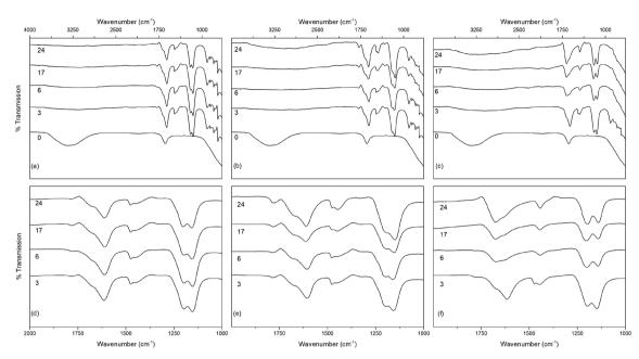
Fig. 7 The infrared spectra of undoped titania treated solvothermally in trifluoroacetic acid for the indicated times at (a)  $100 \,^{\circ}$ C, (b)  $150 \,^{\circ}$ C and (c)  $200 \,^{\circ}$ C, with the corresponding carboxylate stretching regions highlighted in (d–f). Data have been normalised and offset for clarity.
