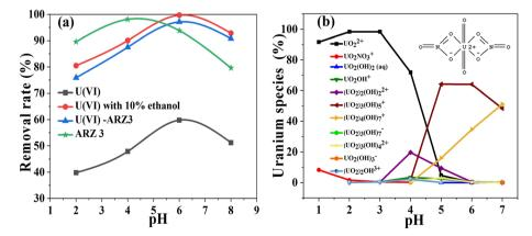
Fig. 5 (a) The effect of pH on the degradation/reduction of 50 mg L<sup>-1</sup> U(vi)-ARZ3, free ARZ3 dye, and free U(vi) ions using the Co@TiO2-C photocatalyst for 60 min (solution volume; 10 mL, catalyst weight; 10 mg) and (b) speciation of uranium in aqueous solution at different pH values.
