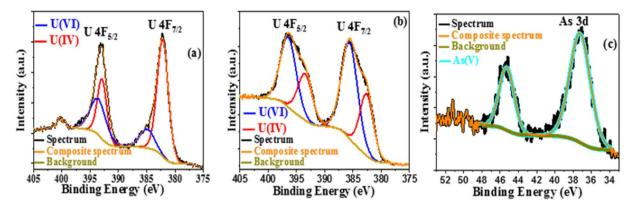
Fig. 9 (a) U 4f XPS spectra in 10% ethanol and (b and c) U 4f and As 3d XPS spectra of the U(v1)-AZR3 complex.
