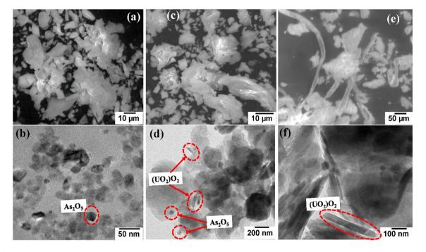
Fig. 10 (a and b) SEM and TEM images of the ARZ3 degraded product. (c and d) SEM and TEM images of uranium and the arsenazo III degraded product. (e and f) SEM and TEM images of the uranium degraded product in ethanol media.
