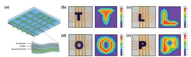
Fig. 5 Spatial pressure distribution based on the sensor array. (a) Schematic diagram of the  $4 \times 4$  sensor array. (b-e) Placement of 3D letters T, L, O and P on the sensor matrix. On the left side there is the actual shape, while on the right there is the capacitance mapping.
