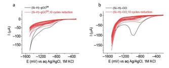
Fig. 6 Electrochemical reduction of gGO and GO (Hummers method). Ten consecutives cyclic voltammograms for the electrochemical reduction of (a) Si-gGO and (b) Si-GO (Hummers' method) in 0.1 M phosphate buffer solution at pH 7.4, and a scan rate of 50 mV  $\rm s^{-1}$ . The potential is presented in mV vs. Ag/AgCl, 1 M KCl. The reduction wave is centred around - 950 mV for both carbon-2D materials. In both systems, the charge decreases by 80-90% after 10 cycles.
