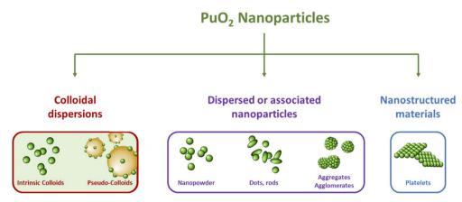
Fig. 2 Scheme illustrating the diversity of PuO<sub>2</sub> nanoparticles reported in the literature with their classification into three subcategories.
