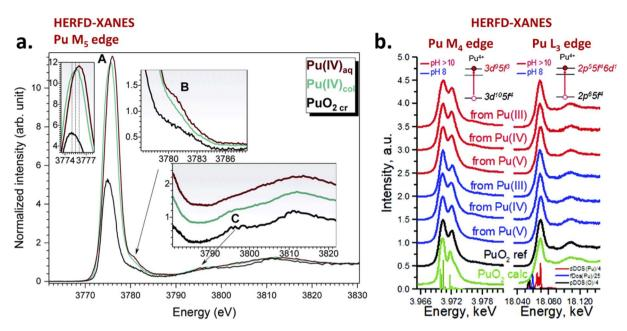
Fig. 19 (a) HERFD-XANES spectra acquired at the Pu  $M_5$  edge for aqueous Pu(v) containing 6% Pu(v), bulk  $PuO_2$  and Pu(v) colloids. Adapted from Vitova et al. 124 with permission from the Royal Society of Chemistry, copyright 2018. (b) HERFD-XANES spectra acquired at the Pu M₄ edge for PuO<sub>2</sub> nanoparticles prepared by the addition of ammonia to Pu(IIII-V) agueous solutions. Adapted from Gerber et al. 111 with permission from the Royal Society of Chemistry, copyright 2020.
