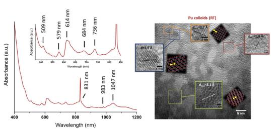
Fig. 4 Left: UV-vis-NIR absorption spectrum acquired on intrinsic Pu(v) colloids prepared by dilution in pure water of a Pu(v) aliquot previously stabilized in nitric medium (RT, [Pu] = 9.2 mM). The spectrum shows the additional presence of Pu(v) absorbing at 830 nm as a mixture with the colloids. Right: HR-TEM image acquired on intrinsic Pu(v) colloids. Adapted from Dalodiere PhD thesis. 97
