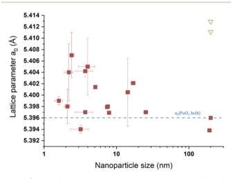
**Fig. 12** Survey of the size vs. lattice parameters extracted from the literature for  $PuO_2$  nanoparticles. The blue line corresponds to the theoretical  $a_0$  value expected for  $PuO_{2.00}$  ( $a_0=5.396$  Å) according to ref. 45. The green triangles transcribe values taken from the literature for aged  $PuO_2$  samples prepared by thermal conversion of oxalate precursors at  $600\,^{\circ}\text{C.}^{138}$  200 nm has been used as an arbitrary value for the 4 points given for this size.
