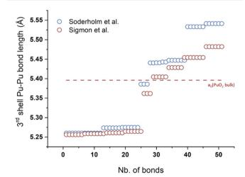
Fig. 13 Pu–Pu bond distances occurring at a distance close to the  $a_0$  parameter extracted from the resolved Pu<sub>38</sub> cluster published by Soderholm *et al.* and Sigmon *et al.* <sup>16,85</sup> The red line corresponds to the theoretical  $a_0$  value given for PuO<sub>2</sub> bulk.
