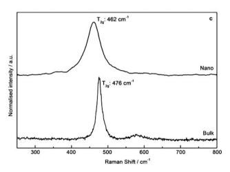
Fig. 9 Raman spectra (488 nm, 1 mW) acquired on  $PuO_2$  nanoparticles (top) and bulk (bottom) in the solid state demonstrating the enlargement and red shift of the  $T_{2g}$  band as evidence of nanoscale materials. Adapted from ref. 117 with permission from John Wiley and Sons, copyright 2014.
