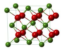
Fig. 11 Cell of the PuO<sub>2</sub> structure. Pu<sup>4+</sup> and O<sup>2-</sup> are shown in green and red, respectively. In the structure, each O is surrounded by 4 Pu atoms forming tetrahedral sites and each Pu is coordinated by 8 O atoms forming infinite arrays of PuO<sub>8</sub> cubes.
