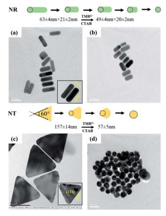
Fig. 6 TEM images of AuNRs (top) and AuNTs (bottom) (left, a and c) before and (right, b and d) after interaction with TMB<sup>2+</sup>.
