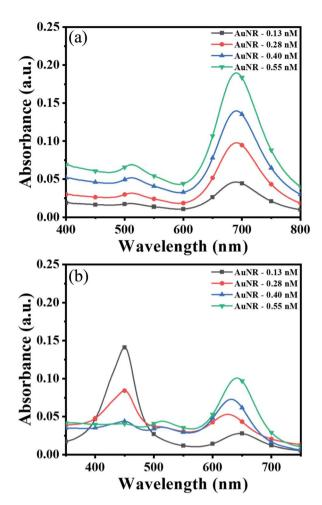
Fig. 3 UV-Vis spectra of (a) AuNRs of 0.13, 0.28, 0.40 and 0.55 nM after interaction with 150  $\mu L$  of water and (b) 150  $\mu L$  of 50  $\mu M$  conc. of TMB $^{2+}$  (for all the samples, total volume was made up to 250  $\mu L$  with water).
