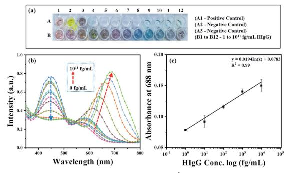
Fig. 7 (a) Photos of microtiter plate wells containing AuNRs interacted with TMB<sup>2+</sup>, produced as a product of the enzymatic reaction in developed competitive p-ELISA and (b) UV-Vis absorption spectra of AuNRs after interaction with different concentrations of HIgG (0 to 10<sup>11</sup> fg mL $^{-1}$ ). (c) The linear relationship between absorbance change ( $\lambda_{max} = 688$  nm) and log concentration of HIgG.
