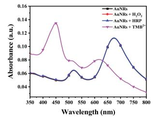
Fig. 4 UV-Vis spectra AuNRs interacted with DI water (black curve),  $H_2O_2$  (red curve), HRP (blue curve) and  $TMB^{2+}$  (pink curve) to study the effect of different reagents on  $TMB^{2+}$  mediated oxidation of AuNRs. (Note: black, blue and red curves are difficult to discern due to overlapping).
