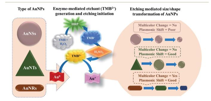
Scheme 1 Schematic illustration of etching-based p-ELISA strategy developed by employing gold nanospheres (AuNSs), gold nanorods (AuNRs), and gold nanotriangles (AuNTs). The enzyme horseradish peroxidase (HRP) hydrolyses 3,3',5,5'-tetramethylbenzidine (TMB) into TMB+, which is oxidized into TMB<sup>2+</sup> upon H<sub>2</sub>SO<sub>4</sub> acid treatment. TMB<sup>2+</sup> acts as an etchant for the gold nanoparticles and leads to their size and shape transformation.
