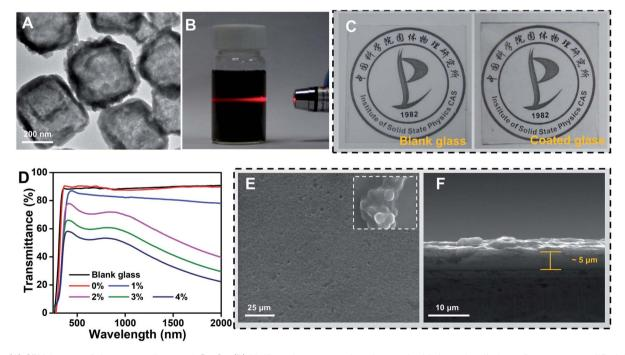
Fig. 2 (A) SEM image of the water-dispersed  $Cu_7S_4$ . (B) Uniform beams can be observed with laser irradiation of aqueous modified  $Cu_7S_4$ / organo-silicone sol solution. (C) Pictures of blank glass and coated glass. (D) Transmittance of photothermal glass with different nanoparticle doping concentrations. (E) and (F) SEM images of photothermal coating with 0.2 wt% doping concentration of  $Cu_7S_4$  photothermal nanoparticles.
