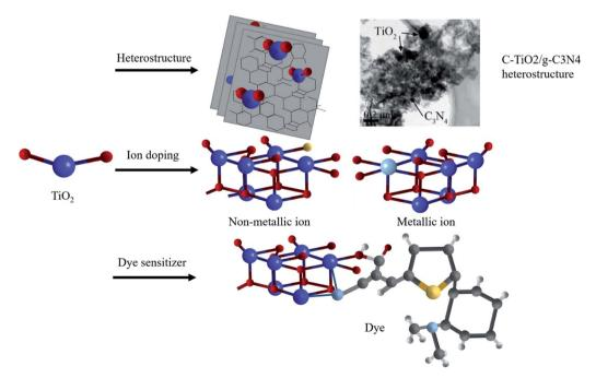
Schematic illustration of modification methods: heterostructures, 52 ion doping and dye sensitization. Copyright 2017 Elsevier.
