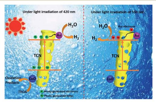
Fig. 16 Two distinct schemes of electron transfer over TCN/CoO/Au at 420 and 550 nm. Reprinted from ref <sup>156</sup>. Copyright 2020 Wiley.
