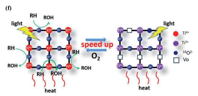
Fig. 10 (a) Experimental diagram of photo(thermal)catalytic degradation of  $CH_3CHO$ . (b)—(e) Photo(thermal)catalytic degradation rate of  $CH_3CHO$ . (f) Mechanism diagram of surface lattice oxygen of  $TiO_2$  participating in the photothermal catalytic oxidation reaction. Reprinted from ref. 123.
