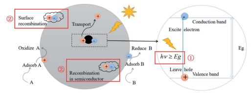
Schematic illustration of semiconductor photocatalysis and its two most important restraining factors.
