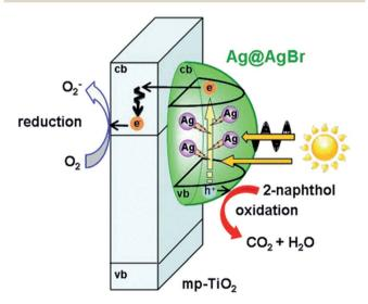
Fig. 7 Action mechanism of the Ag@AgBr/mp-TiO $_2$  photocatalyst under visible-light irradiation. Reproduced from ref. 101. Copyright 2016, ACS.
