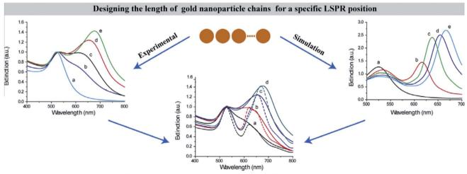
"Trial and error" fit of the experimental data with a linear combination of numerical simulations
