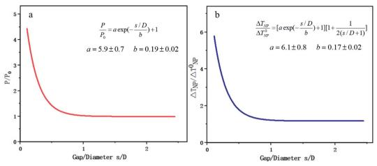
Fig. 13 Plasmon coupling of double Au NPs based on COMSOL. (a) Scaling law of light absorption power and relative particle spacing. (b) Scaling law of steady state temperature and relative particle spacing. Reproduced from ref. 145.
