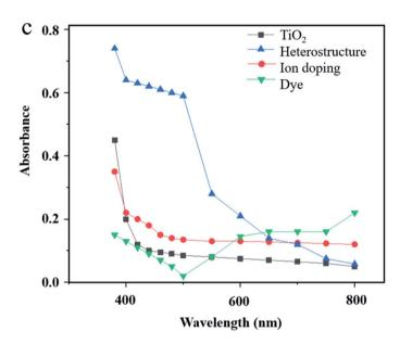
Fig. 6 Expanding the optical response range by adjusting the energy band structure. (a) Light absorption mechanism of dye sensitization as an example. (b) Energy band structure of different modification methods. (c) Comparison of the light absorption efficiency of typical modification examples. Reproduced with data source from ref. 51, 71 and 74.
