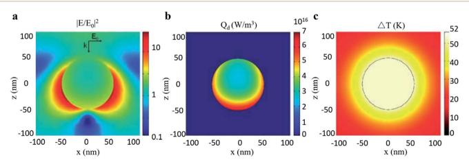
Fig. 14 Photothermal effect of a gold sphere with 50 nm radius in water. (a) Electric field intensity normalized to the incident field. (b) Heat power volume density  $Q_0$ , (c) Steady-state temperature increase due to 530 nm light excitation. Reprinted from ref <sup>30</sup>. Copyright 2012 American Chemical Society.
