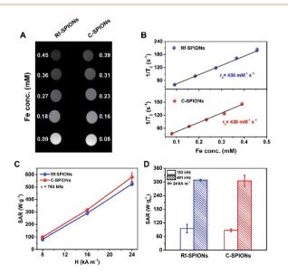
**Fig. 6** (A)  $T_2$  weighted MR phantom image of the SPIONs. (B) Plot of  $T_2^{-1}$  versus Fe concentration for Rf-SPIONs (blue) and C-SPIONs (red) in water. (C) SAR values as a function of the applied magnetic field at a frequency of 763 kHz for the SPIONs. (D) SAR values of the SPIONs were measured at frequencies of 163 and 491 kHz under a constant magnetic field strength of 24 kA m $^{-1}$ .
