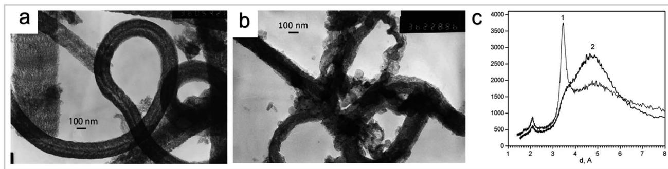
Fig. 7 (a) Typical electron image of CNF obtained by a CVD method from acetylene on the Fe/C/SiO<sub>2</sub> catalyst. (b) Typical electron image of CNF activated melted KOH modified with 2 wt% of copper. (c) XRD patterns of CNF (curve 1) and CNF activated with melted KOH (curve 2) "reproduced from ref. 34 with permission from Elsevier, copyright 2008".
