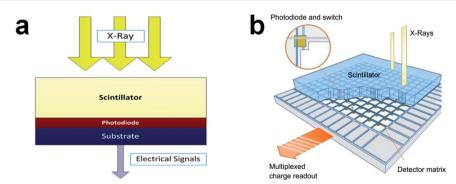
Fig. 1 (a) Schematic depiction of the three main functional layers in a common X-ray CT detector. Reproduced with permission.<sup>34</sup> Copyright 2013 Springer Nature Limited. (b) Schematic description of an X-ray flat detector constituted by columnar CsI:Tl<sup>+</sup> scintillator and a detecting matrix of amorphous-silicon photodiodes. Reproduced with permission.<sup>18</sup> Copyright 2013 Elsevier.
