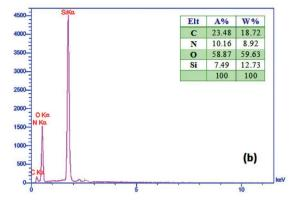
EDX spectra of the obtained PMAMOS using precursor I prepared in THF (a) and DMF solvents (b).
