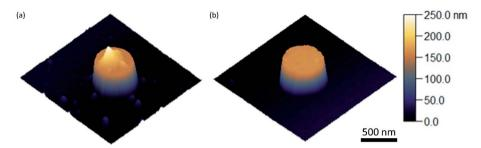
Fig. 4 AFM height mapping;  $1.5 \times 1.5 \,\mu\text{m}^2$  maps. (a) AFM image of a single cylinder with a thick layer of QDs stamped on top. The print is nonuniform and incomplete. (b) AFM image of a single cylinder with a monolayer of QDs stamped on top. The print is uniform and complete.
