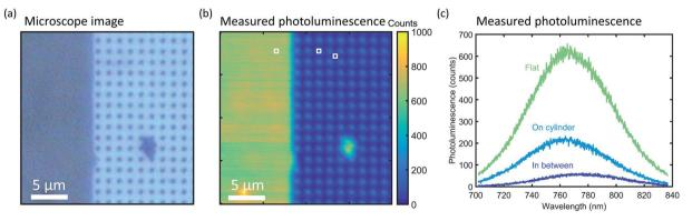
Fig. 3 Photoluminescence mapping after thick QD print. (a) Microscope image of the Si substrate (blue) with a thick QD layer on top of flat Si and the Si cylinder array (gray). (b) PL map of the area depicted in (a). Color scale depicts the intensity at 760 nm wavelength. (c) PL spectra of three typical positions on the sample, indicated by the squares in (b): on the flat Si (green), in the middle of a cylinder (light blue), and in between four cylinders (dark blue).
