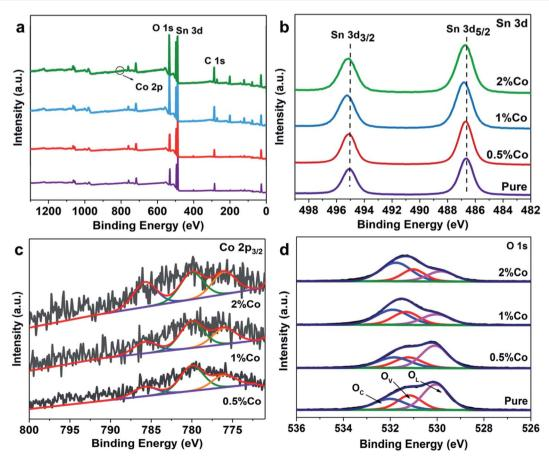
Fig. 2 (a) XPS survey spectra, (b) Sn 3d spectra, (c) Co 2p<sub>3/2</sub> spectra and (d) O 1s spectra of the pure and Co-doped SnO<sub>2</sub> NPs.
