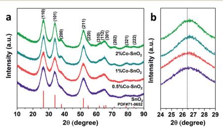
Fig. 1 (a) Full angle range of XRD patterns and (b) high-resolution of (110) peak of the pure, 0.5%, 1% and 2% Co-doped SnO<sub>2</sub> NPs.
