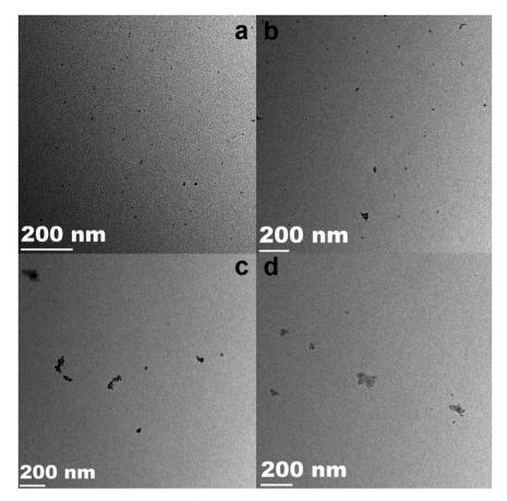
Fig. 3 (a-d) The TEM images of SnO<sub>2</sub> NPs, 0.5%Co-SnO<sub>2</sub> NPs, 1%Co-SnO<sub>2</sub> NPs and 2%Co-SnO<sub>2</sub> NPs
