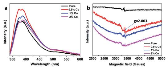
Fig. 12 (a) Photoluminescence spectra and (b) electron paramagnetic resonance spectra of SnO<sub>2</sub> NPs, 0.5%Co-SnO<sub>2</sub>, 1%Co-SnO<sub>2</sub> and 2%Co-SnO<sub>2</sub>.
