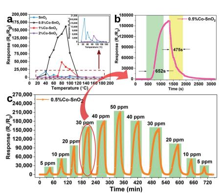
Fig. 6 (a) Response curves of four samples to 30 ppm formaldehyde at 20-180 °C and their partial enlargement (inset), (b) the response and recovery curves of the  $0.5\%\text{Co-SnO}_2$  NPs at 90 °C to 30 ppm formaldehyde, (c) the response transients of the  $0.5\%\text{Co-SnO}_2$  NPs at 90 °C and different formaldehyde concentration.
