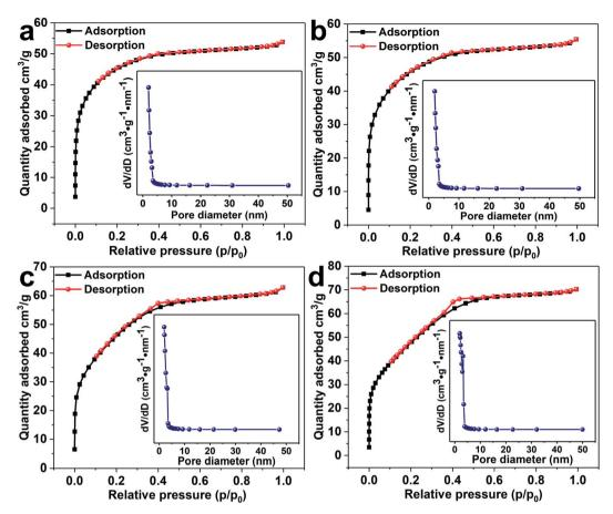
Fig. 5 Nitrogen adsorption—desorption isotherms and corresponding pore size distribution (inset) of (a) SnO<sub>2</sub> NPs, (b) 0.5%Co-SnO<sub>2</sub> NPs, (c) 1% Co-SnO<sub>2</sub> NPs and (d) 2%Co-SnO<sub>2</sub> NPs.
