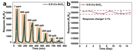
Fig. 7 (a) The response transients of 0.5%Co-SnO<sub>2</sub> NPs to ultra-low concentrations of formaldehyde, (b) long-term stability of 0.5%Co-SnO<sub>2</sub> NPs to 30 ppm formaldehyde at 90 °C.
