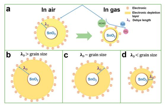
Fig. 11 (a) The cross-sectional view of the sensing mechanism of SnO<sub>2</sub> NPs in the presence of air and in formaldehyde; schematic of SnO<sub>2</sub> NPs grain size versus electron depletion layer thickness, (b) electronic depletion layer ( $\lambda_D$ ) > grain size, (c) electronic depletion layer ( $\lambda_D$ ) ~ grain size, (d) electronic depletion layer ( $\lambda_D$ ) < grain size.
