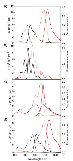
Fig. 3 UV/Vis/NIR absorption spectra (dashed lines) as well as the fluorescence spectra (solid lines) of the neutral (black) and dianionic (red) (a) **PBI–CI**, (b) **PBI–H**, (c) **PBI–Ph** and (d) **PBI–OPh** measured in DCM ( $c_0 = 4 \times 10^{-4}$  M for absorption,  $c_0 = 1 \times 10^{-5}$  M for fluorescence of PBI and  $c_0 = 1 \times 10^{-4}$  M for fluorescence of PBI<sup>2-</sup>) at room temperature using TBAHFP (0.1 M) as electrolyte.
