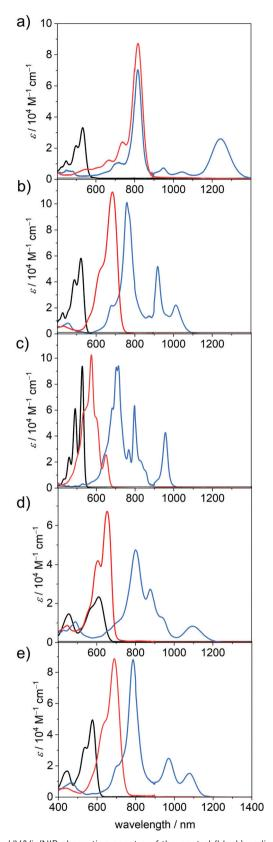
Fig. 2 UV/Vis/NIR absorption spectra of the neutral (black), radical anionic (blue) and dianionic (red) PBI species of (a) PBI-ClCN, (b) PBI-Cl, (c) **PBI-H**, (d) **PBI-Ph**, and (e) **PBI-OPh** measured in DCM ( $c_0 = 4 \times 10^{-4}$  M) at room temperature using TBAHFP (0.1 M) as electrolyte.
