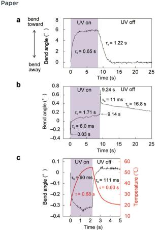
Fig. 6 Bending of enol-1b crystals (Movie S5, ESI†). (a) Thin (171  $\times$  17.2  $\times$ 2.4  $\mu m^3$ ), (b) slightly thick (2410  $\times$  191  $\times$  65.5  $\mu m^3$ ), and (c) thick (2030  $\times$  $344 \times 174 \ \mu m^3$ ) crystals bent through photoisomerisation and/or the photothermal effect upon UV laser irradiation of the (100) top face at 960 mW  $cm^{-2}$  (a and b) and 230 mW  $cm^{-2}$  (c).
