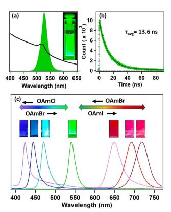
Fig. 2 Optical properties of MAPbBr $_3$  NCs. (a) Steady-state absorption (black) and photoluminescence (PL) spectra (green) of MAPbBr $_3$  NCs. (b) PL transient of MAPbBr $_3$  NCs upon exciting at 405 nm. (c) Tuning the PL through anion exchange by oleylammonium halides (OAmX; X = Cl, Br, I).
