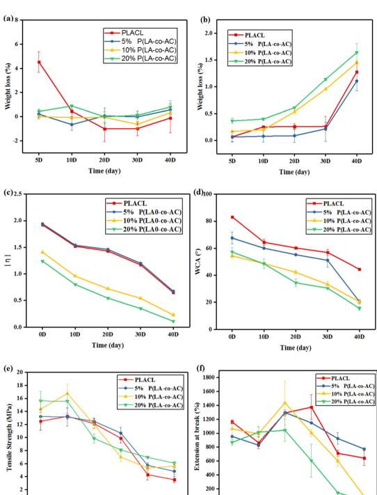
Fig. 5 Degradation properties: (a) weight loss in artificial urine; (b) weight loss in deionized water; (c) intrinsic viscosity; (d) WCA change; (e) tensile strength; and (f) extension at break.
