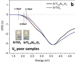
Fig. 11 Surface photovoltage (SPV) spectra of SrTiO<sub>3</sub> (blue) and SrTi<sub>0.9</sub>Al<sub>0.1</sub>O<sub>3</sub> (black) (a) V<sub>O</sub> rich made by heating profile 1 and (b) V<sub>O</sub> poor made by heating profile 2, respectively. CPD values under illumination are reported relative to the dark. The band-like onset was approximated by linear extrapolation (red dash). The inset pictures show the appearance of the respective films used for SPV measurement.
