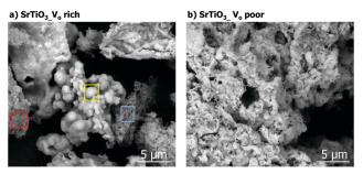
Fig. 5 SEM image of (a) V<sub>O</sub> rich SrTiO<sub>3</sub> made with heating profile 1 and (b) V<sub>O</sub> poor SrTiO<sub>3</sub> made with heating profile 2.
