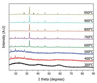
Fig. 2 Ex situ powder X-ray diffraction patterns of the calcined sample for the synthesis of SrTiO<sub>3</sub> at various temperatures. TiO<sub>2</sub> impurity peaks are marked with asterisks (\*).
