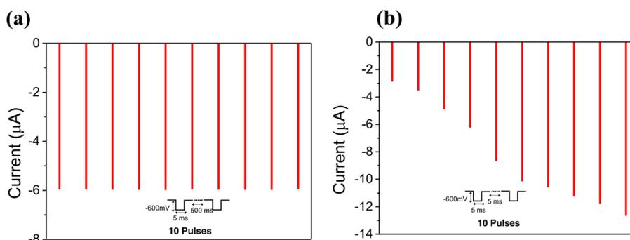
**Fig. 11** Mimicking the spike-timing dependent plasticity (STDP) using a MemPVCell-1 device for 10 identical applied pulses ( $-600$  mV of amplitude, 5 ms of duration) of (a) 500 ms and (b) 5 ms interval.
