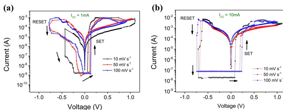
Fig. 4 Influence of the scan rate and compliance current on resistive switching of MemPVCell-1. Switching memristive characteristics of MemPVCell-1 by sweeping the dc bias from  $-1$  to  $1$  V at different scanning rates ( $10 \text{ mV s}^{-1}$ ,  $50 \text{ mV s}^{-1}$ ,  $100 \text{ mV s}^{-1}$ ) and compliance current applied [ $1 \text{ mA}$  (a) and  $10 \text{ mA}$  (b)].
