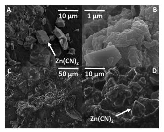
Fig. 1 SEM images of the LDPE/Zn(CN)<sub>2</sub> interfaces on the fracture surfaces of composites (A) (C-40-0), (B) (C-20-2.5), (C) (C-40-10), and (D) (C-40-10). Note the superior integration of the Zn(CN)2 crystallites into the LDPE matrix, indicated by rounded edges, when an sufficient amount of ionic liquid is present
