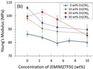
Fig. 3 Young's modulus for LDPE/Zn(CN)<sub>2</sub>/[EMIM][TFSI] composites. (a) Young's modulus slightly increases with the concentration of Zn(CN)2, (b) that slightly decreases with [EMIM][TFSI]. Lines are provided to guide the eye. Error bars represent the standard deviation of measurements on replicate samples
