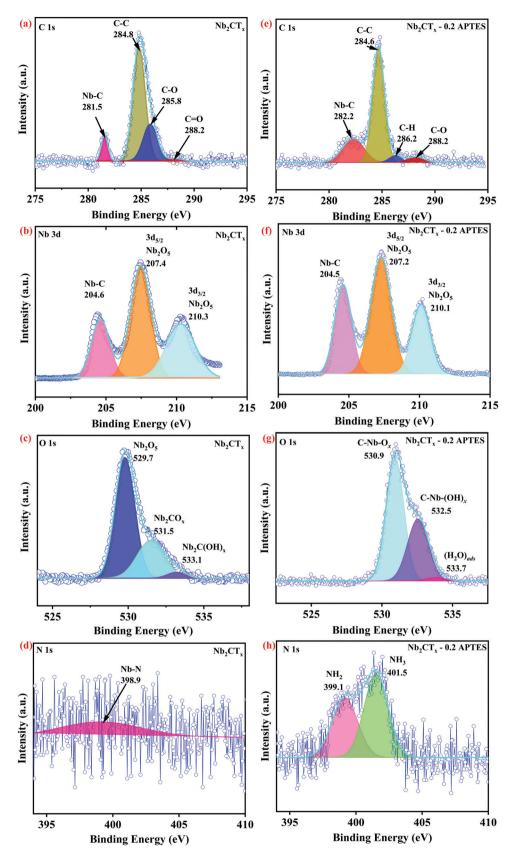
Fig. 2 XPS results of the as-synthesized Nb<sub>2</sub>CT<sub>x</sub> MXene (a–d) and Nb<sub>2</sub>CT<sub>x</sub>-0.2 APTES MXene (e–h).
