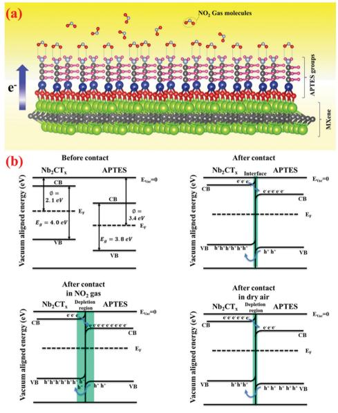
Fig. 9 (a) Sensing mechanism of Nb<sub>2</sub>CT<sub>x</sub>-0.2 APTES MXene for NO<sub>2</sub> gas, (b) energy band diagram of the Nb<sub>2</sub>CT<sub>x</sub>-0.2 APTES interface.
