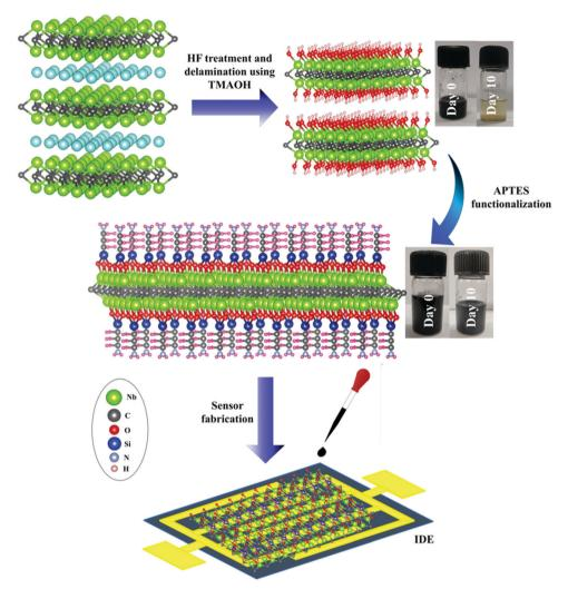
Fig. 1 Schematic representation of synthesis and sensor fabrication of Nb<sub>2</sub>CT<sub>x</sub> and Nb<sub>2</sub>CT<sub>x</sub>-APTES MXene
