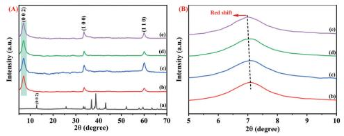
Fig. 3 (A) Full and (B) enlarged XRD of the Nb<sub>2</sub>AlC MAX Phase (a), Nb<sub>2</sub>CT<sub>x</sub> MXene (b), Nb<sub>2</sub>CT<sub>x</sub>-0.1 APTES (c), Nb<sub>2</sub>CT<sub>x</sub>-0.2 APTES (d), Nb<sub>2</sub>CT<sub>x</sub>-0.3 APT€ (e).
