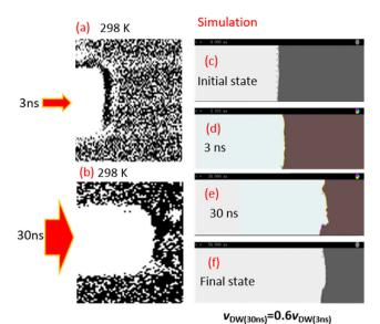
Fig. 4 Polarized optical microscope images of current-driven domain wall (DW) shape at room temperature for (a) 3 ns, and (b) 30 ns pulse duration width. Simulation results of DW shape, (c-f) for 3 ns and 30 ns pulse duration width.
