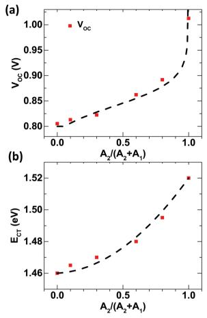
Fig. 2 Alloy composition vs. (a) changes in  $V_{\rm OC}$  using the double-diode model (the dotted line represents the fitting of experimental  $V_{\rm OC}$  values with eqn (2)) and (b) changes in the  $E_{CT}$  value of the BHJ alloy composition determined from sensitive EQE studies (the dotted line represents the fitting of experimental  $E_{CT}$  values with eqn (3).
