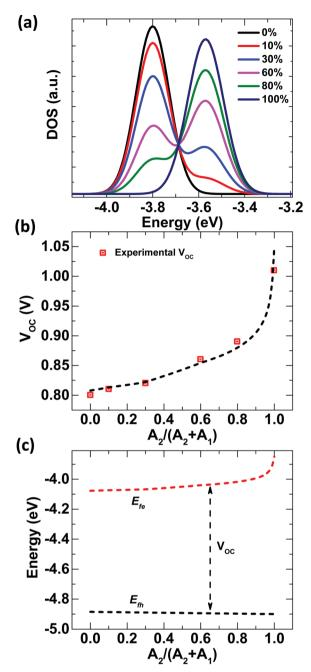
Fig. 3 Changes in DOSs for different A<sub>1</sub>:A<sub>2</sub> concentrations plotted against energy using eqn (2) and eqn (3); (b) experimental  $V_{OC}$  values (red squares) fitted with a population occupancy DOS model (dashed line); and (c) QFL splitting for different A1: A2 ratios in D ternary blend solar cells, obtained from population occupancy in a Gaussian disorder model
