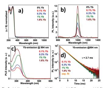
Fig. 8 (a) Absorption spectra, (b) PL spectra, (c) PLE spectra, and (d) PL decay dynamics of Yb doped  $Cs_2AgInCl_6$  double perovskite MCs. Reproduced with permission. 77 Copyright 2019, American Chemical Society.
