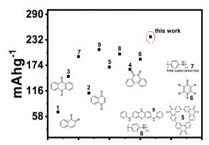
Fig. 9 Comparison of the specific capacitancse of the reported organic cathodes for the zinc battery.
