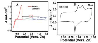
Fig. 3 (A) Voltammogram of zinc and pheno@cnt showing the cell voltage of 1.19 V. (B) Voltammogram showing the excellent stability of the electrode in 100 multiple sweep cycles at a 50 mV s $^{-1}$  scan rate.
