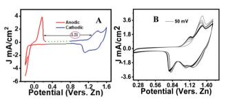
Fig. 2 (A) Cyclic voltammograms of zinc and neat phenothiazine showing the output cell voltage of 1.21 V. (B) Multiple voltammograms show the poor stability during multiple scans (cyclic voltammograms of the neat phenothiazine-coated glassy carbon electrode as the working and zinc plate as the counter and reference electrodes in 2 M ZnSO<sub>4</sub>).
