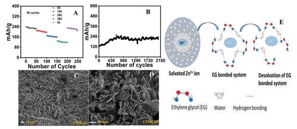
Fig. 8 (A) Rate stability test (fifty continuous cycles have been shown for each current density). (B) Prolonged cycling experiment for 2200 cycles at a current density of 300 mA  $g^{-1}$ . Pheno@CNT in aqueous 2 M ZnSO<sub>4</sub>-ethylene glycol (1:1) electrolyte. (C and D) FESEM images of the anode and cathode surfaces after cycling. (E) Cartoon illustrating the solvated Zn<sup>2+</sup> ions as well as the ethylene glycol-associated solvation-desolvation mechanism.
