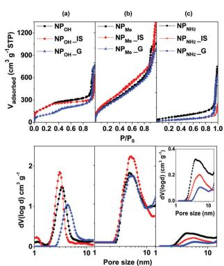
Fig. 1  $N_2$  adsorption/desorption isotherms at 77 K (above) and the corresponding pore size distribution calculated using the NLDFT method (below) of the hybrid MSNs, both IS and G, in comparison to the related complex-free silica nanoparticles (NP): (a) NP<sub>OH</sub>, (b) NP<sub>Me</sub>, and (c) NP<sub>NH2</sub>.
