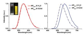
Fig. 4 Emission spectra at room temperature of NP<sub>Me</sub>\_IS (left, red) and NP<sub>Me</sub>\_G (right, blue) in the solid state (dotted line) and in water suspension (solid line). Inset: photograph of the aqueous suspension of NP<sub>Me</sub>\_IS under visible and UV  $\lambda_{\rm exc}$  370 nm illumination.
