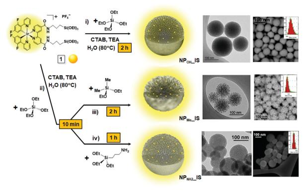
Scheme 1 Schematic representation of the synthesis of *in situ* hybrid mesoporous organometallo-silica nanoparticles (NP<sub>OH</sub>\_IS, NP<sub>Me</sub>\_IS and NP<sub>NH2</sub>\_IS), including TEM and SEM images of each, showing their textural differences, as well as their DLS size distributions.
