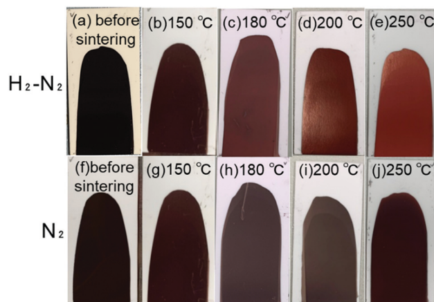
Fig. 7 Digital images of the surface of the sintered copper nanoparticle layers. (a) Before sintering, (b–e) sintered at various temperatures indicated in the image under 3% \text{H}_2 - \text{N}_2 gas flow, (f) before sintering, (g–j) sintered at various temperatures under nitrogen gas flow.
